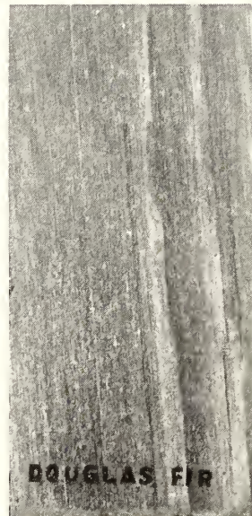
FIGURE 2-39.—Split tangential surfaces of Sitka spruce and Douglas-fir showing the "pocked" appearance of the spruce, not found in Douglas-fir. This characteristic is most pronounced in Sitka spruce with narrow rings and is almost entirely absent in very wide-ringed material.
